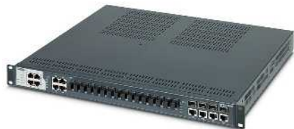
8 RJ45-Ports, 4 Gigabit-Combo-Ports (SFP oder RJ45) und 16 LWL-Ports (Multimode)
